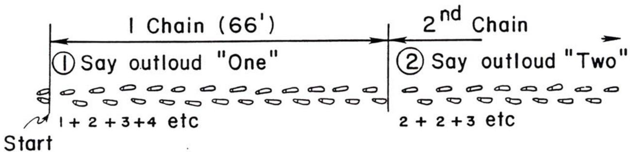
If your land is hilly, you'll want to practice this on steeper ground as well. In this case you must be sure to lay off the 66-foot distance horizontally and not along the slope. This may require measuring the 66 feet in several shorter horizontal segments - called "breaking chain" by surveyors.
