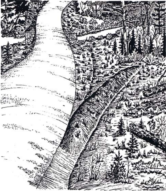
Figure 1. Diversion ditch. Divert road drainage into undisturbed vegetation so that it does not directly enter the stream.
